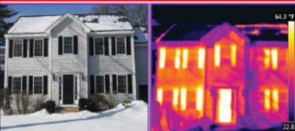
Identify air leaks and problems in your home with thermal imaging
